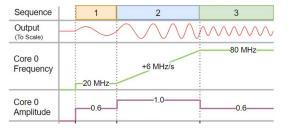
Above, the example sequence of three commands for a single core, shows a fixed 20 MHz frequency with 60% amplitude in step 1, a 10 seconds frequency ramp with 6 MHz/s slope and full 100% am-
